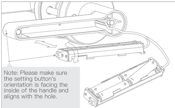
Note: Please keep the setting needle safe as it is used to set many functions on the handle. If you lose this, it is possible to use a paperclip to push the set button.
